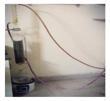
Fig. 2: Overall view of extraction using Soxhlet apparatus.
